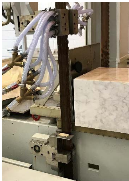
Figure 7. Bandsaw with upper hydrostatic guides and lower bearing guides
