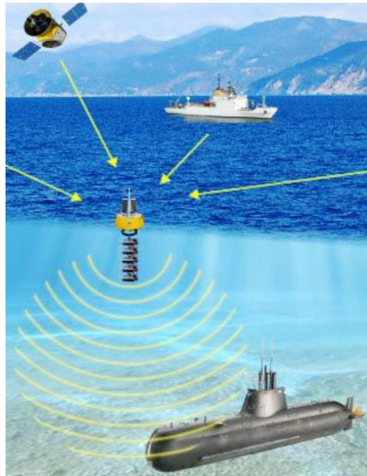
Figure 2. Wireless (acoustic) buoyant GNSS-like UPS. Application of JANUS [10].
