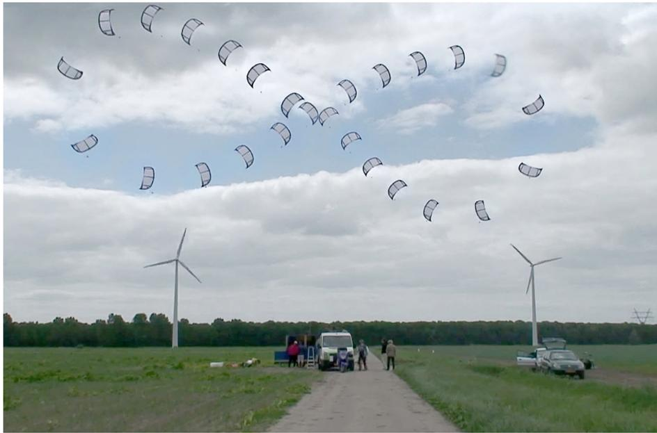
**Figure 2.** Composite photo of a crosswind figure-of-eight maneuver ( $\Delta t = 1$  s) of a tube kite with 25 m<sup>2</sup> surface area [7].
