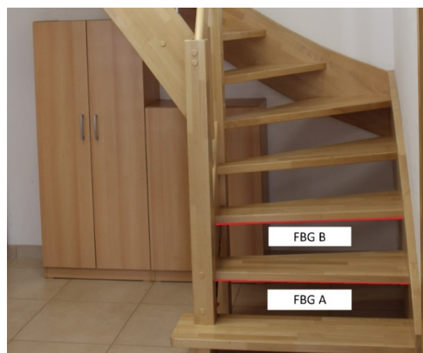
Fig. 4: Placement of FBG sensors on the staircase in the smart home (SH), room R104.
