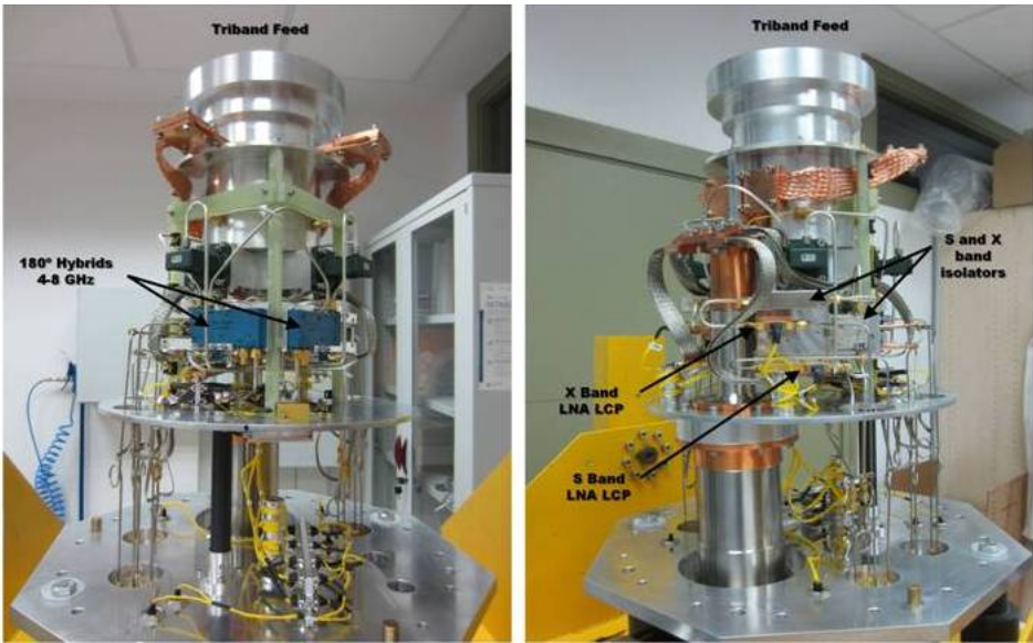
Figure 8. Receiver components inside de cryostat.
