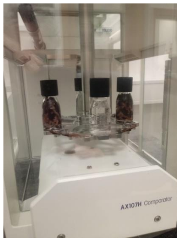
Figure 4: Two experimental and two control test tubes on Mettler-Toledo AX107H Comparator
