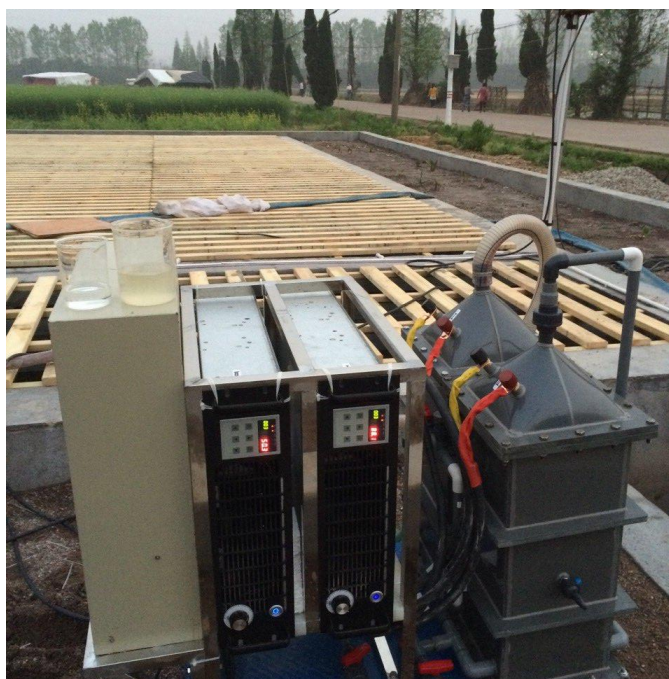
Fig. 4 Wastewater treatment unit by electrocoagulation and electrooxidation
