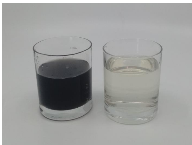
Fig. 3 Wastewater before (left glass) and after (right glass) treatment with electrokinetics
