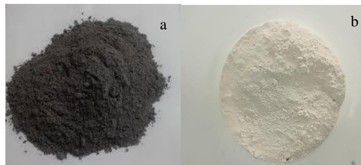
Figure 1. Pictures of raw materials: (a) olive-pine bottom ash (OPBA) after sieving stage, and (b) metakaolin after calcination step.
