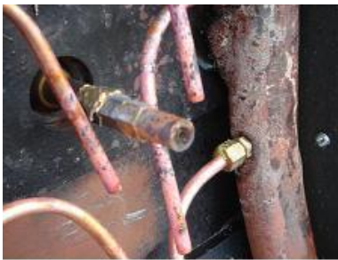
(c) Melting-down of Torches(2 ea) due to heat-blocking of frame
