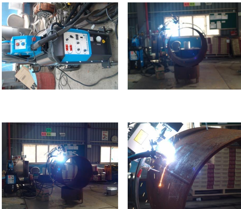
Figure 8. Orbital Welding Test
