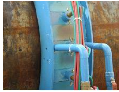
(b) Discoloration of Frame due to overheating
