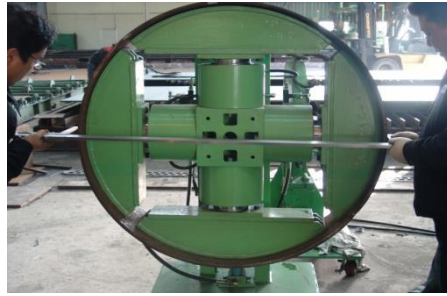
(e) Measuring of deformation after test
