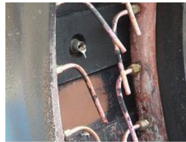
(c) Melting-down of Torches(2 ea) due to heat-blocking of frame
