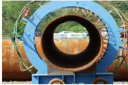
(c) Heating and Water Cooling of Tube
