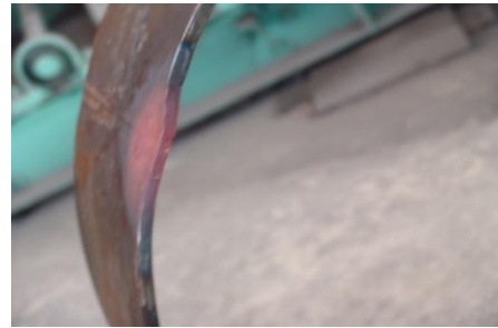
(b) Steel tube after correction of outside surface
