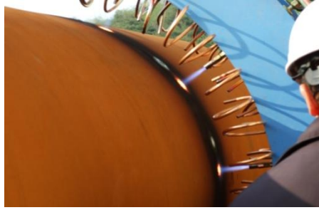
(e) Details in heating and water cooling of Tube
