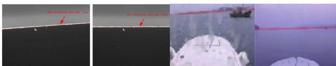
Figure 7. Sea-sky detection based on haar wavelet decomposition
