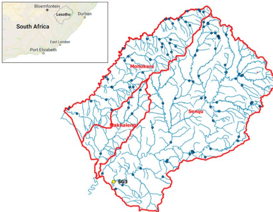
Figure 1. Map of Lesotho. Lesotho's catchment boundaries are shown in red, hydrographic network in blue, flow monitoring stations are the blue dots, and the pertinent hydrometric station SG3 (highlighted in yellow) [28].
