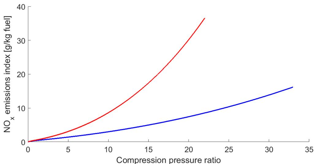
**Figure 7.** NO<sub>x</sub> emissions index for the SSBJ (red) and for the long haul subsonic airline (blue).
