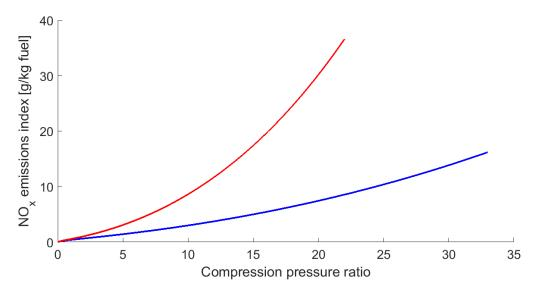
**Figure 7.** NOx emissions index for the SSBJ (red) and for the long haul subsonic airline (blue).
