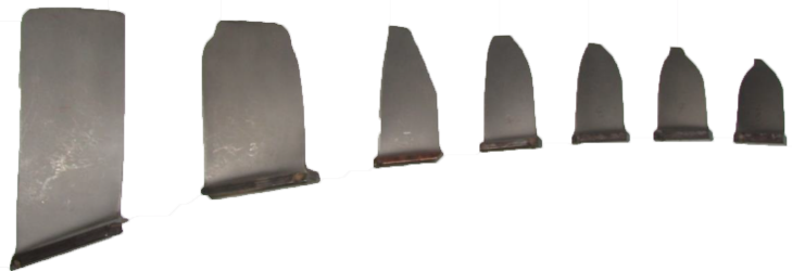
Figure 2. Blades of a compressor of a turboshaft subjected to erosive wear
