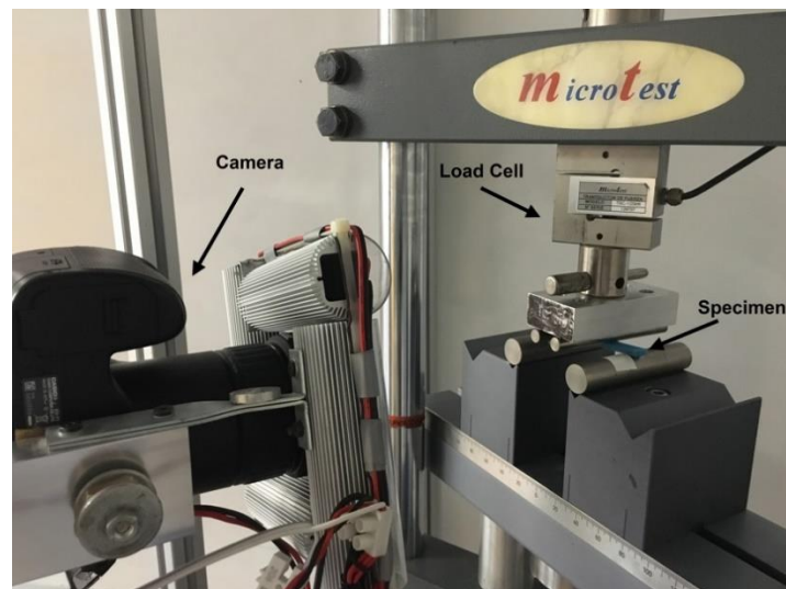
Figure 6. The installation used to perform the 4 points bending tests.
