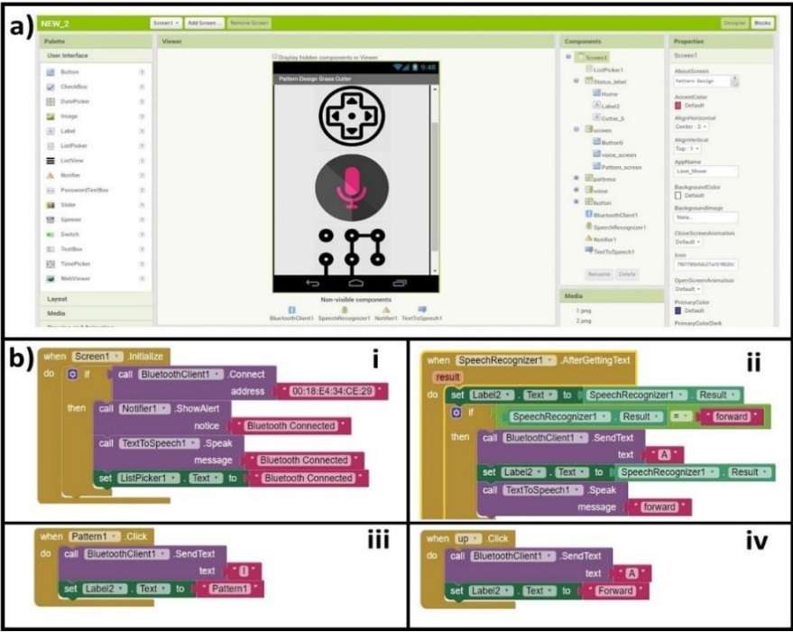
Figure 4. Design view and Blocks editor of Android Application for pattern design grass cutter. (a) Design view window. (b) i. Bluetooth module component. ii. Speech recognition component. iii. Send text component for the pattern. iv. Send text component for up arrow button.
