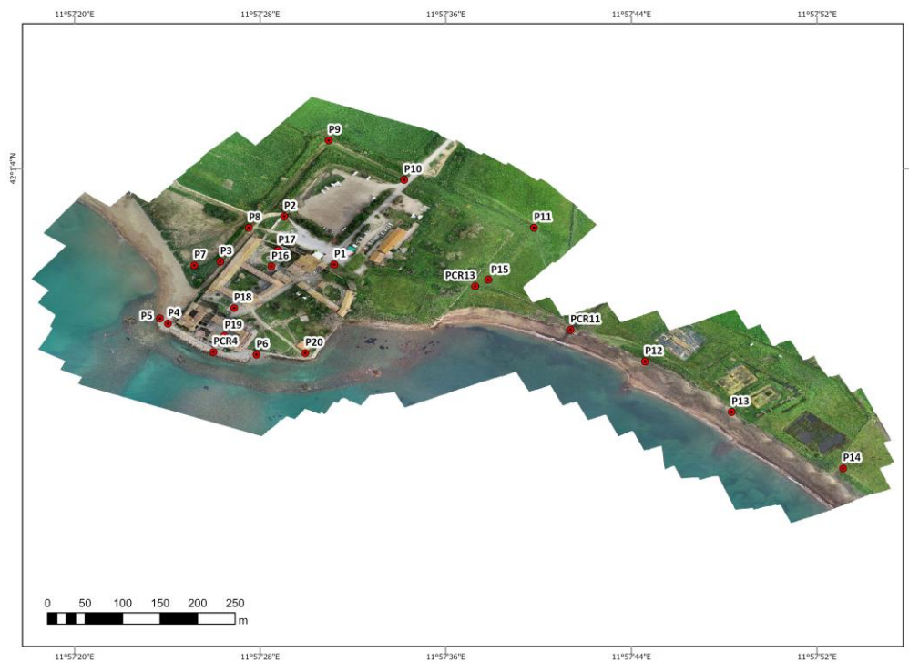
Fig.2 The orthophoto with the Ground Control Points (red dots) position used during the UAV surveys.
