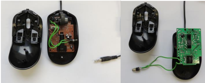
Figure 10 (left) and Figure 11 (right): Modified computer mouse with extra connection to the left mouse button.
