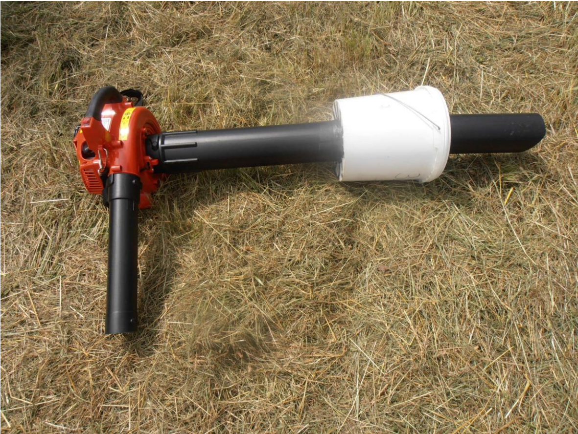
Figure A5 The leaf vacuum, after modification, used to collect arthropods in the Hockgraben grassland area. Arthropods are collected in a mesh bag positioned in the bucket, where airflow is reduced due to the larger volume
