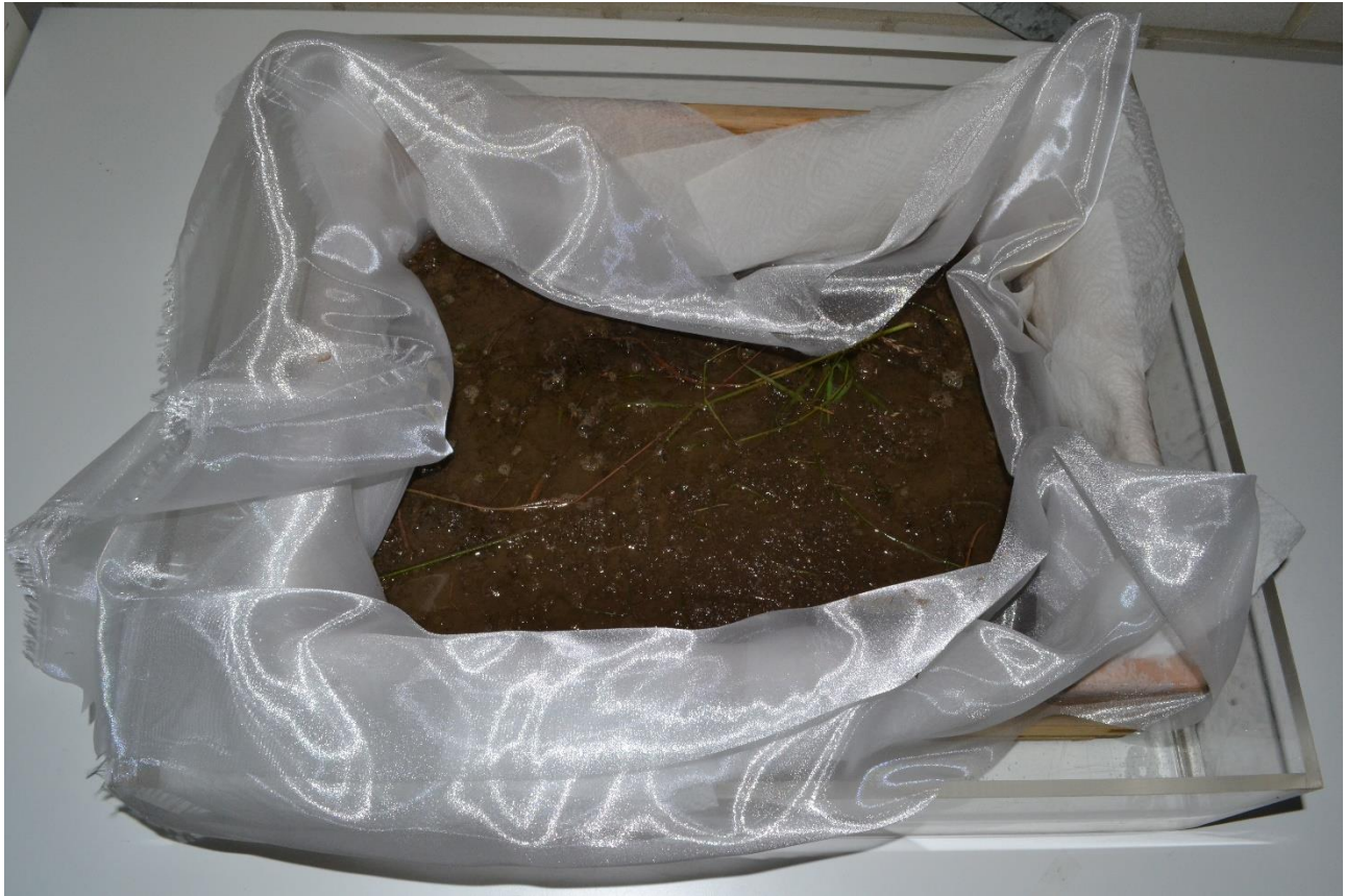
Figure A4 Soil during nematode extraction. The soil was placed in a sieve, above a layer of kitchen paper and a layer of fine meshed fabric, and then covered with water. Nematodes will reach the bottom of the tray going through the fine meshed fabric and the other layers.
