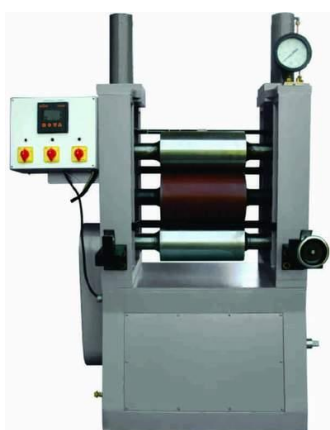
Figure 11. Laboratory calendering machine PE7006 (Premier Enterprise, India).
