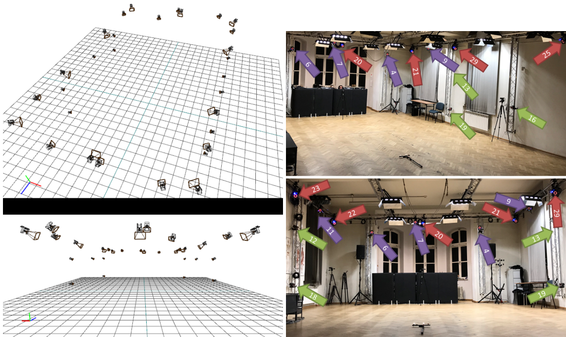
Figure 8. Camera locations: a) Schematic view in Vicon Blade software, b) actual setup in HML. Color denotes camera series: violet – Vantage, green – Bonita, red – T40
