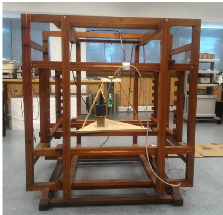
Figure 3. Image of the triaxial arrangement of Helmholtz coils used in this project
