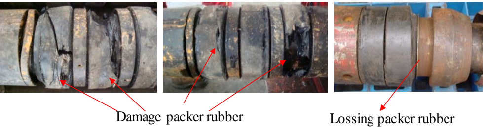
Fig.2 Failure cases of rubber packer
