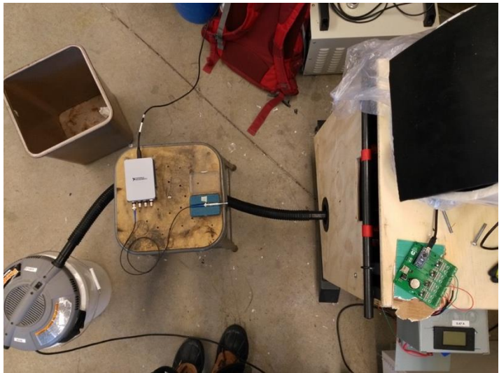
Figure 7: Sound measurement test setup depicting the microphone in one of the test locations
