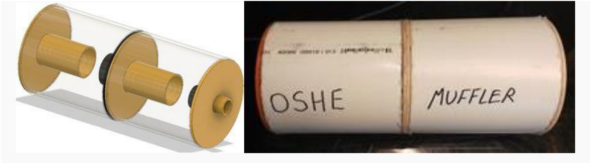
Figure 9: Comparison between CAD of chamber and finished expansion chamber.
