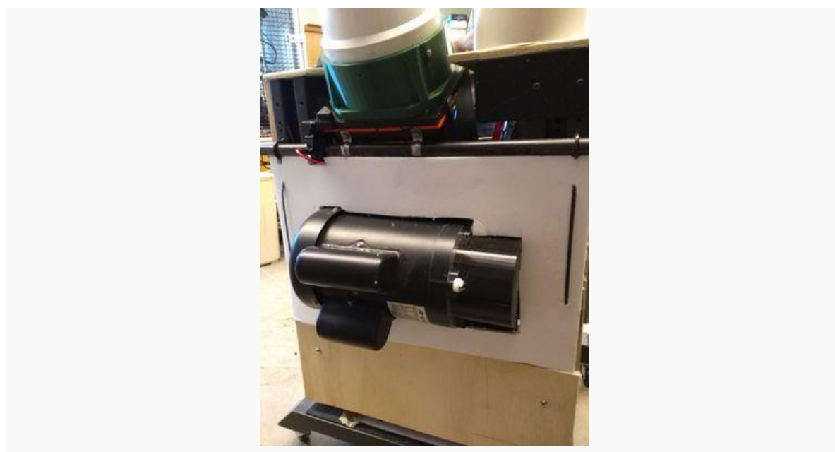
Figure 8: Granulator panel gaps filled with sound proofing material
