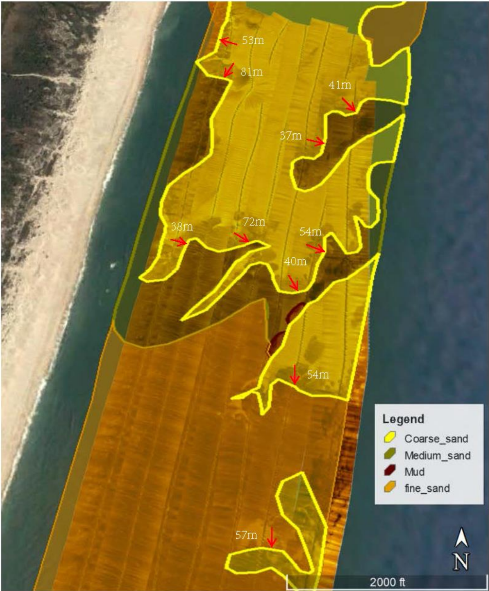
Figure 19: Temporal changes in sediment class boundaries, Assateague Island National Seashore, Maryland. The profile in the bottom is the side-scan sonar mosaics collected during May 2015. Shaded polygons on the top represent sediment classes inferred from the side-scan sonar mosaics collected during October 2015. Please note the west-south-eastward shift (38 - 57 m) in the boundaries of fine - coarse sand sediment classes.
