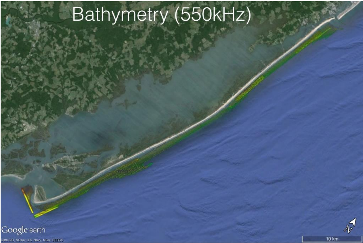
319 320 Figure A7. Bathymetry mosaic (1m/pixel) from 2014-2015 acoustic surveys (550 kHz) for the entire 321 study area. Notable features captured in the bathymetry included pronounced shore-attached 322 oblique bars. 323 Resulting swath bathymetry data for the study side was gridded to a resolution of 1m/pixel. 324 Reliable bathymetry data was obtained for approximately half the total sonar swath width resulting 325 in 50% seafloor coverage in depths ranging from 2 to 12 m. Early sampling in 2014 around Fishing 326 Point was conducted using spacing resulting in 100% bathymetry coverage (200% side-scan sonar) 327 but the survey rate was unsustainable for the entire study site and it was agreed upon by all project 328 partners to expand the line spacing to achieve 100% side-scan and 50% bathymetry. This survey 329 strategy is also in keeping with the same approach used by the USGS in their larger regional 330 coverage provided for a meaningful connection of this study to that regional effort. The resulting 331 swath bathymetric grids extend what was only single-beam echosounder data from the precursor 332 2011 project and thus provide an enhanced baseline for AINS resource managers. Notable 333 features captured in the bathymetry included pronounced shore-attached oblique bars.
