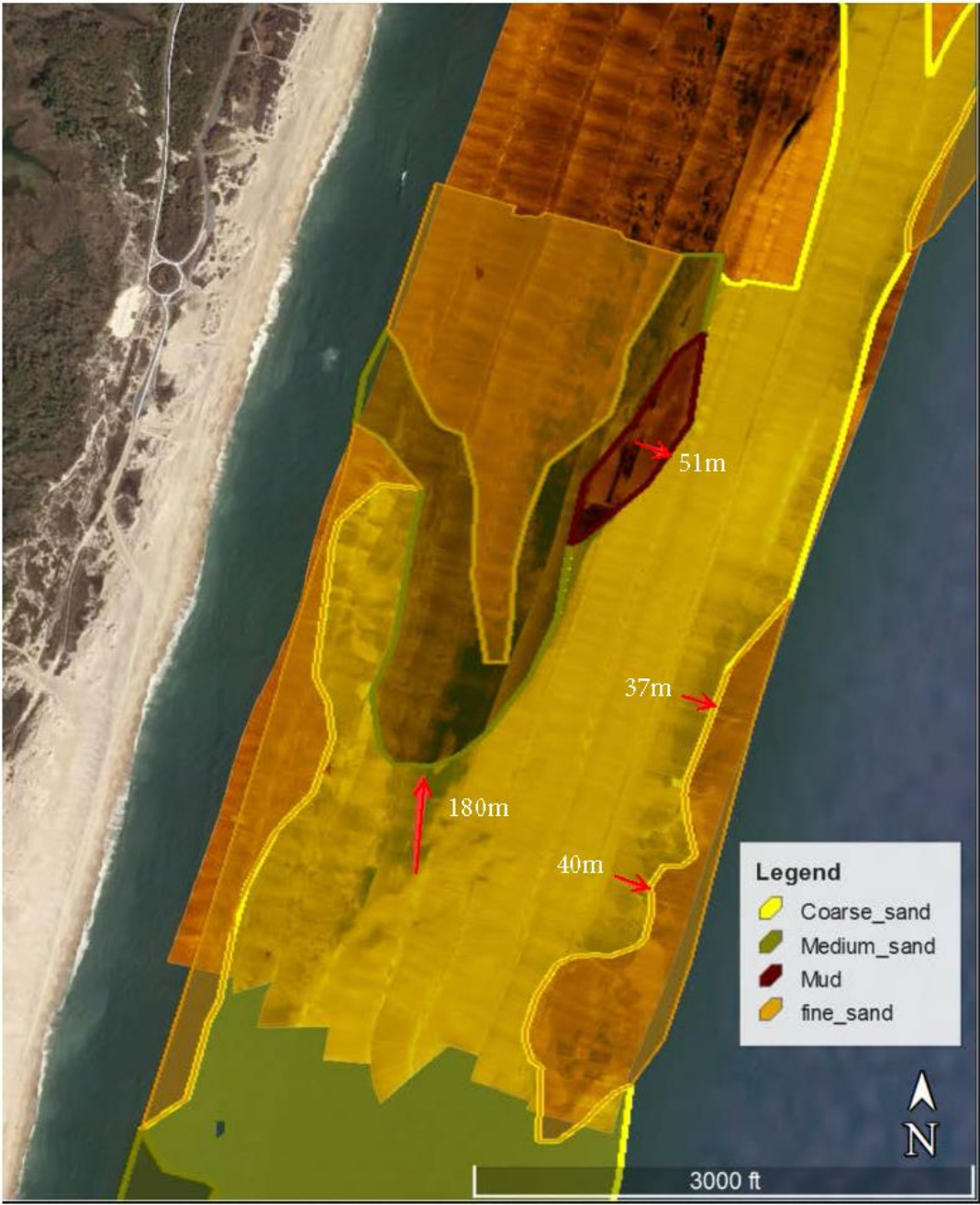
Figure 17: Temporal changes in sediment class boundaries, Assateague Island National Seashore, Maryland. The profile in the bottom is the side-scan sonar mosaics collected during May 2015. Shaded polygons on the top represent sediment classes inferred from the side-scan sonar mosaics collected during October 2015. Please note the northward shift (180 m) in the boundary of mud-coarse sand sediment class and Southeastward shift (37- 40m) in the boundary of fine - coarse sand sediment class.
