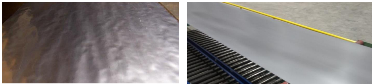
Figure 4. Comparison of martensitic grade surface quality (a) water quenched strip with an oxide layer, steam pockets & off flat errors, and (b) hydrogen quenched strip with clean surface
