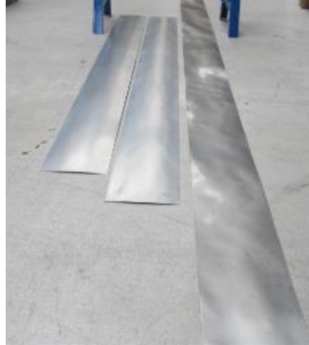
Figure 3. Comparison of martensitic grade flatness by (a) water quenched with edge wave and center buckle and (b) hydrogen quenched strip with excellent flatness (courtesy HyCAL*)
