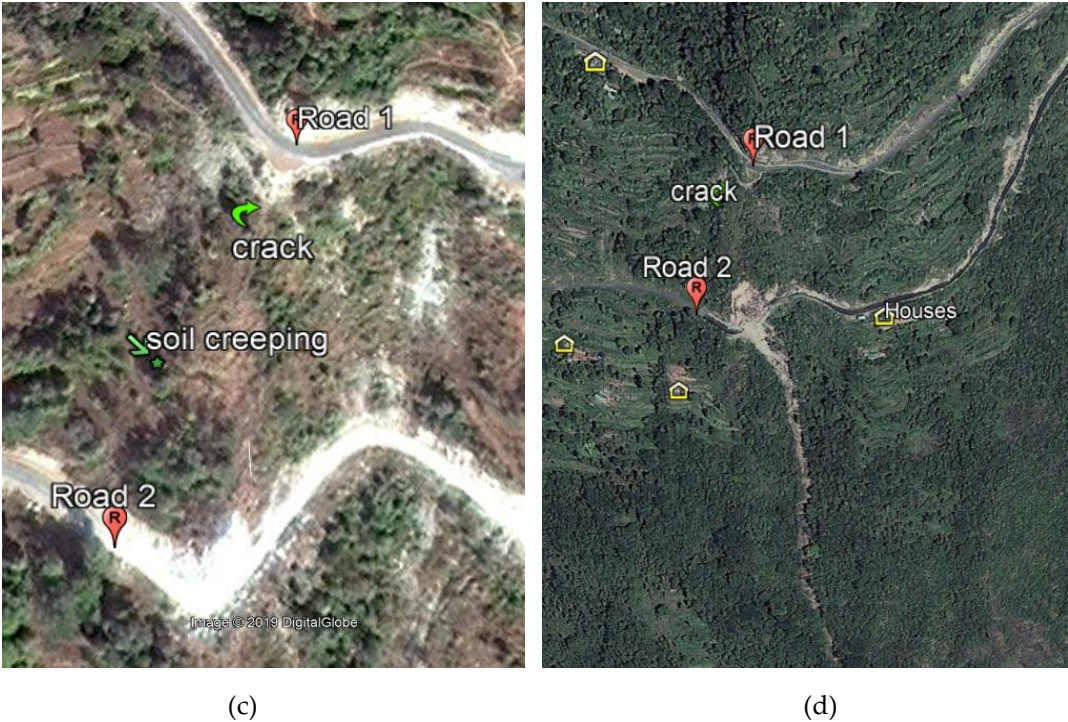
Figure 3. Aerial photographs of the study area: (a) The roadway was not constructed until the year 2006; (b) A few years later in 2009, an earthen road 1 and 2 one above the other was constructed and the minor cracks underneath the road one was observed; (c) After a year in 2010, the flexible pavement was constructed, and slightly enlarged cracks were found with creeping of soil down towards road section two; (d) The failure slope in between two road section during 2011 Sikkim earthquake event.
