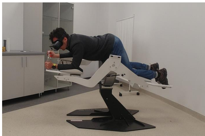
136 137 138 Figure 2. Icaros Pro – flight simulator in VR
