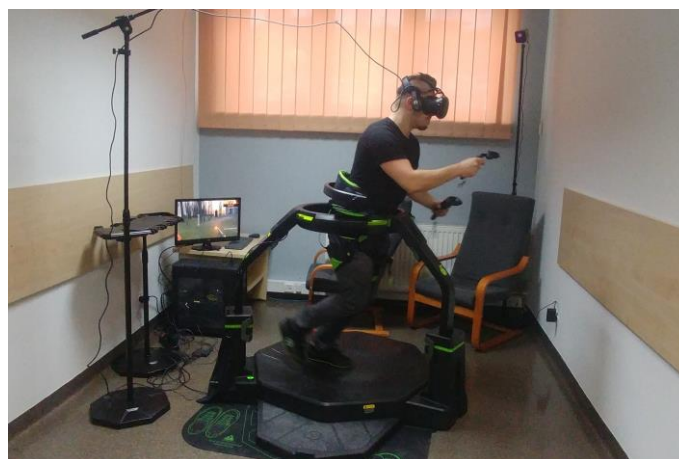
Figure 1. Omni-directional Omni treadmill enabling locomotive movements in VR
