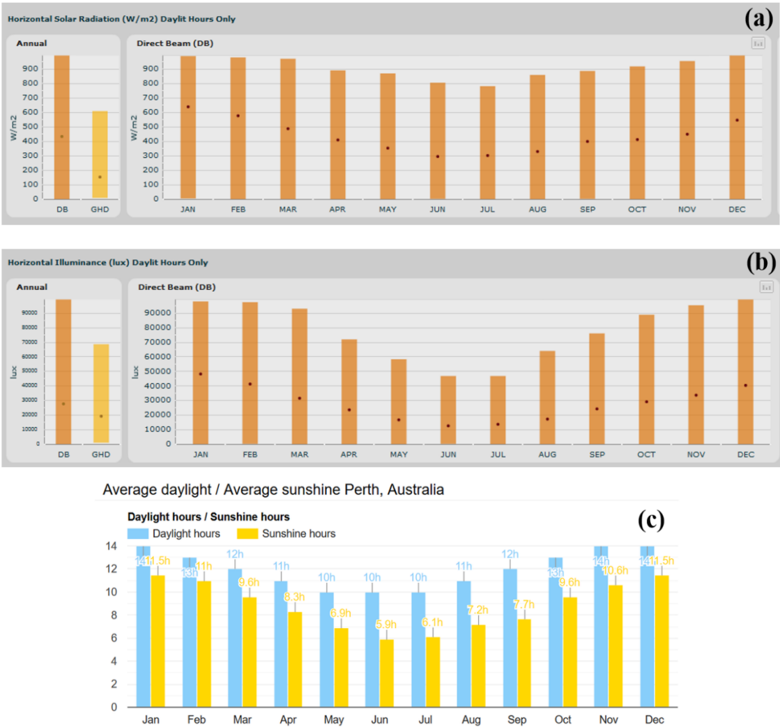
Figure 6. Seasonal yearly climate-related solar irradiation parameter variations for Perth, Australia. (a) Monthly averaged and maximum-recorded direct-beam solar irradiation intensities measured across horizontal plane; (b) monthly averaged and maximum-recorded direct-beam solar illuminance values measured across horizontal plane; (c) monthly distributions of the total daylight hours and the daily sunshine durations. The datasets shown in parts (a) and (b) have been obtained using COMFEN 5 software [45]; the dataset of part (c) has been published online by [31].
