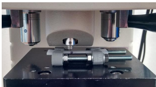
Figure 7: Measurement of microhardness of a deformed polymer subjected to tension.
