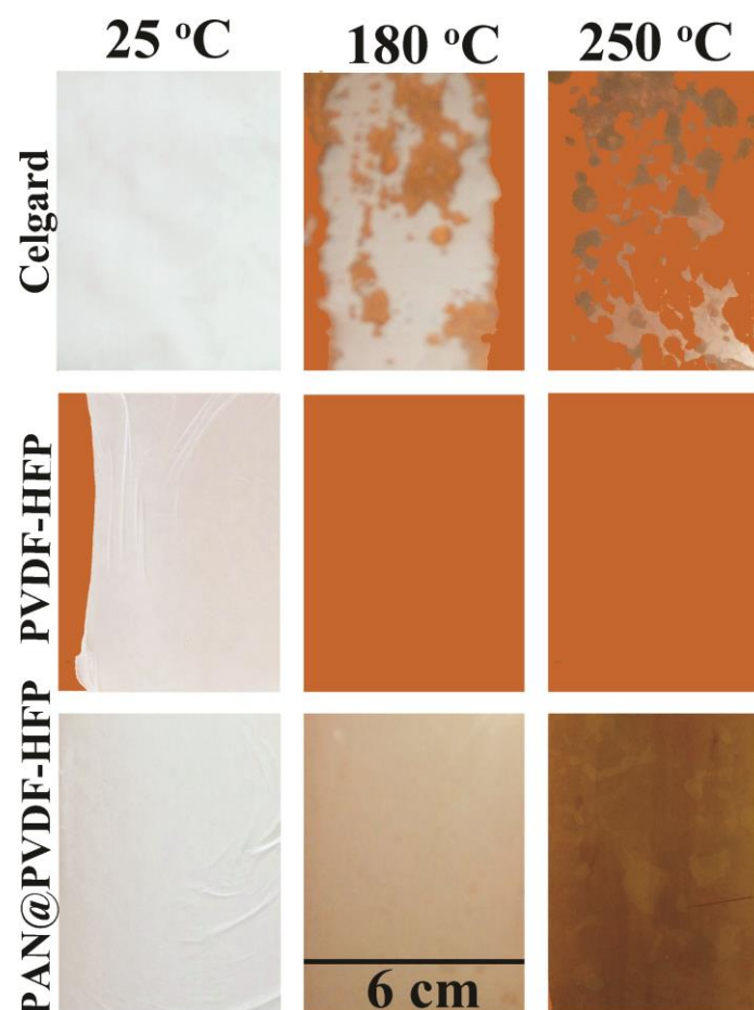
213 Figure 3. The thermal stability tests of commercial Celgard2400 separator, PVDF-HFP and PAN@PVDF-HFP 214 fiber network. 215 216 217
