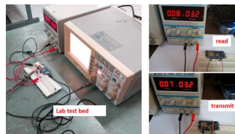
Fig. 9. A lab testbed with the standard device (NodeMCU).
