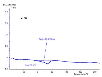
Differential scanning analysis (DSC) of pure o-PDA
