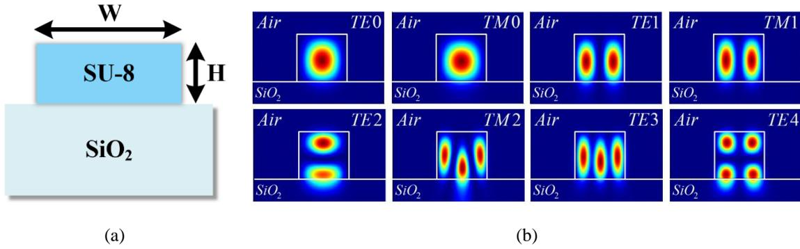
**Figure 2.** (a) Cross-section of the ridge waveguide; (b) E-field profiles of SU-8-based waveguide structure.
