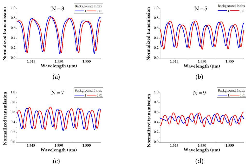
**Figure 6.** Transmission spectrum according to N when the background index of the S-bend resonator is 1 and 1.01: (a) N = 3; (b) N = 5; (c) N = 7; (d) N = 9.
