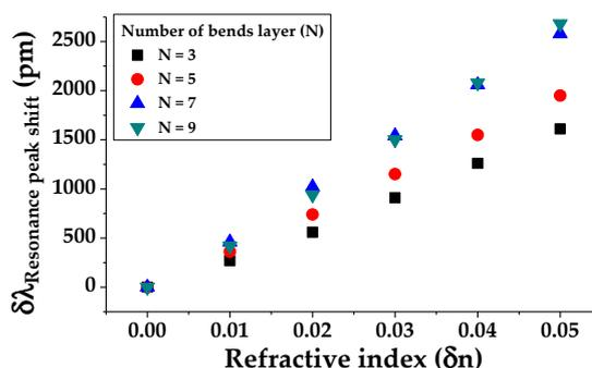
Figure 7. Resonance wavelength peak shift according to N.
