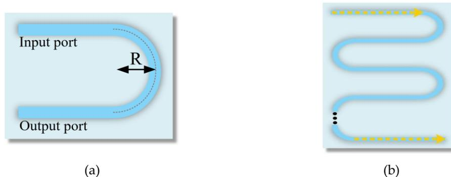
**Figure 3.** (a) Schematic of a semi-circle; (b) The S-bend structure for mode discrimination.
