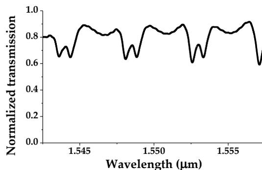
Figure 5. Normalized transmission of S-bend resonator with  $N = 1$ .
