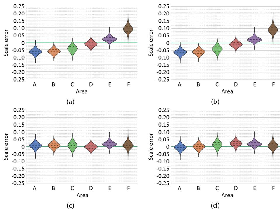
**Figure 24.** Estimated scale errors per segment for model AUTT28: (a/b) Global / Incremental SfM with similarity transformation navigation fusion. (c/d) Global / Incremental SfM with multi-objective BA navigation fusion.
