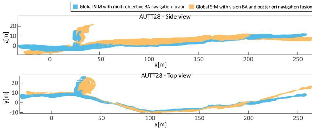
**Figure 25.** Comparison of navigation fusion strategies on the reconstruction of 3D models.
