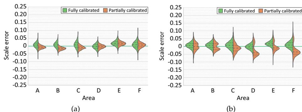
**Figure 29.** Comparison of estimated scale errors computed with fully- and partially-calibrated method using: (a) only nearly-parallel laser pairs; (b) all laser pairs.
