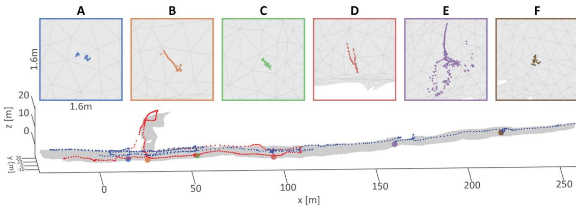
**Figure 23.** 3D reconstruction with the distribution of laser observations per segment for AUTT28 area. Red and blue dots correspond to VICTOR dives 654 and 658.
