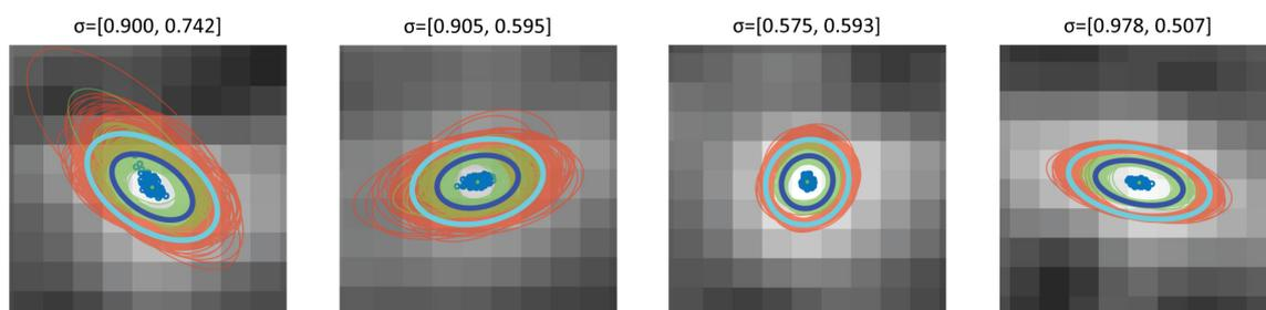
**Figure 10.** Examples of detected laser spot with uncertainty estimated through MC simulation for image shown in Fig. 8. Individual detections and uncertainties are depicted with blue dots and red/green ellipses, while final uncertainty estimate is blue and cyan.
