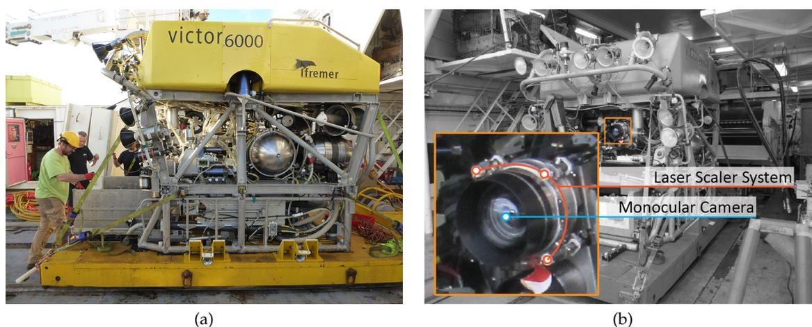
**Figure 11.** (a) ROV VICTOR 6000 (IFREMER) [79]. (b) Enlarged camera and laser system.
