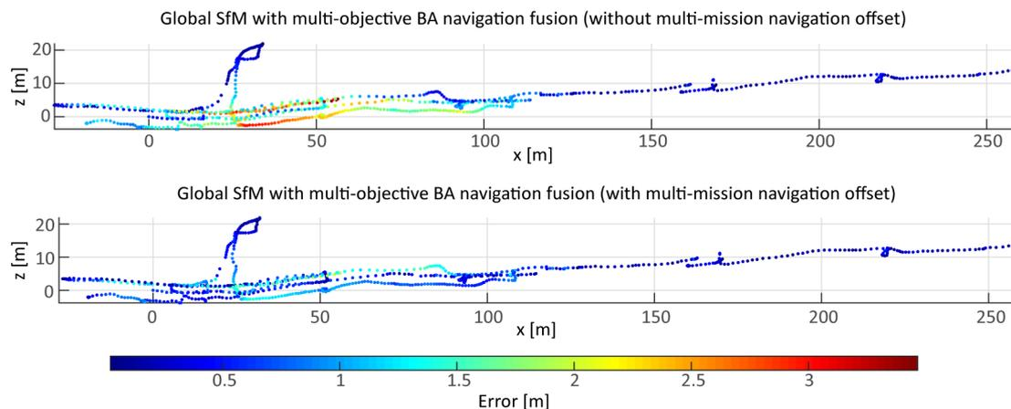
**Figure 26.** Comparison of multi-survey data fusion strategies on the estimated camera path.
