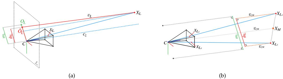
**Figure 5.** Scale estimation using (a) fully-calibrated and (b) partially-calibrated approach, based on the 3D model and optical image depicting the laser beam projection on the scene intersection with the scene.
