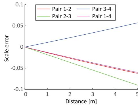
**Figure 19.** Error induced in scale error estimate due to disregarding non-parallelism of laser beams.
