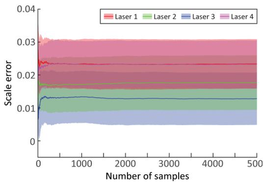
**Figure 18.** Evolution of scale error estimate with increasing number of MC iterations.
