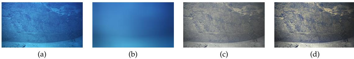
**Figure 2.** (a) Original UW image. (b) Chromatic components  $(\alpha, \beta)$  of the estimated local illuminant. (c) White balanced image. (d) Final enhanced image.
