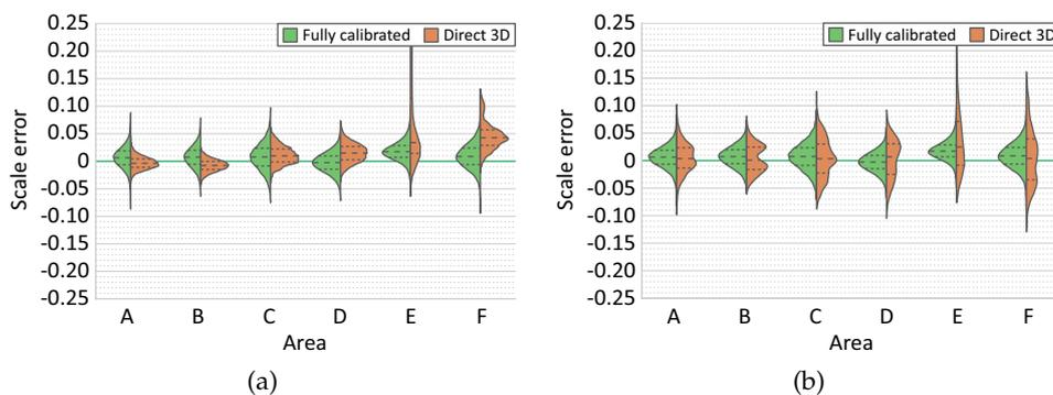
**Figure 28.** Comparison of estimated scale errors computed with fully-calibrated and simplistic direct 3D method using: (a) only nearly-parallel laser pairs; (b) all laser pairs.
