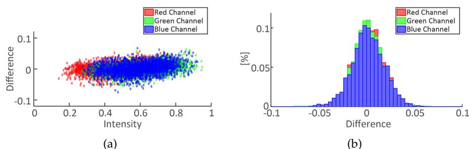
**Figure 9.** Characterization of image noise: (a) image noise vs. pixel intensity; (b) distribution of noise per color channel.
