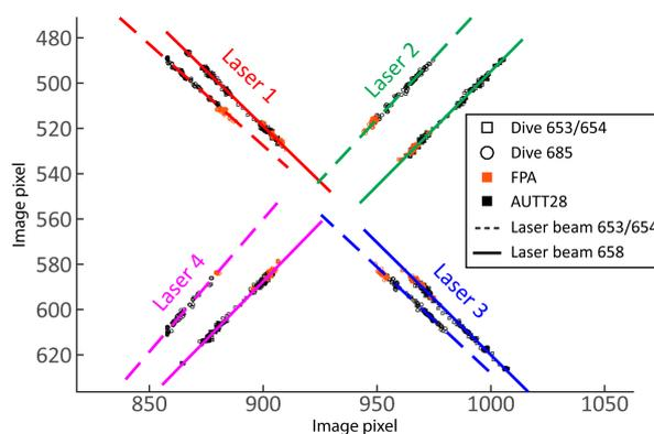
**Figure 16.** Calibration results for dives 653/654 and 658. Solid and dotted lines represent the projections of estimate laser beams on the image plane, while projected laser intersections with the scene are depicts as squares/circles.
