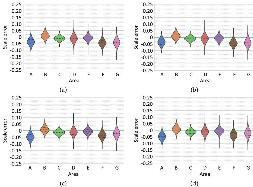
**Figure 22.** Estimated scale errors per segment for model FPA: (a/b) Global / Incremental SfM with similarity transformation navigation fusion; (c/d) Global / Incremental SfM with multi-objective BA navigation fusion.
