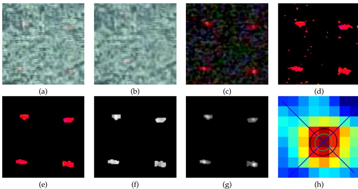
**Figure 8.** Laser spot detection: (a) predicted ROI of original image; (b) aligned auxiliary patch; (c) ROI after the removal of texture information (intensity  $\times 5$ ); (d) potential laser pixels after color thresholding; (e) filtered laser pixels; (f,g) estimated laser beam luminosity without/with texture removal; (h) detected laser spot with detection uncertainty.
