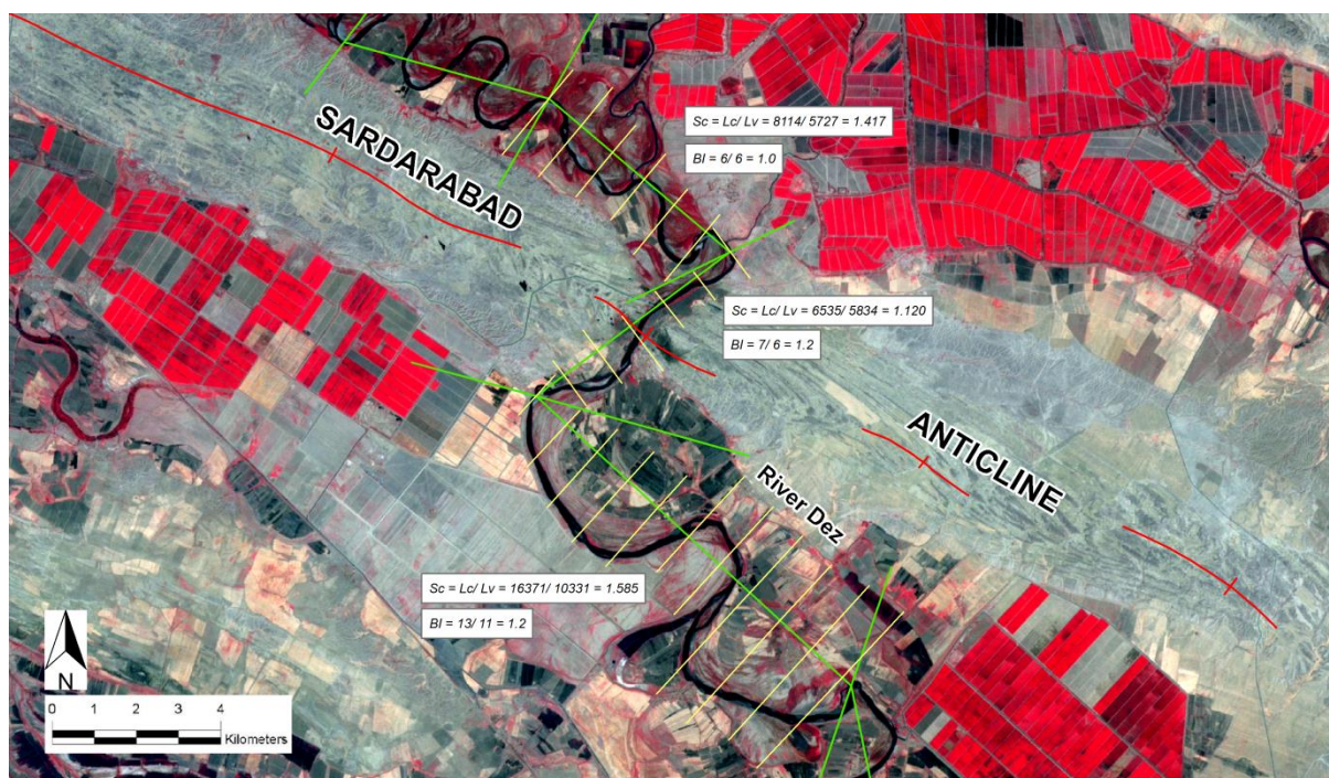
Figure 4 The measurement of Sc and BI (False-colour Landsat image (2001) of the River Dez incising across the Sardarabad Anticline, centred on c. 31^{\circ}57'N 48^{\circ}36'E )
