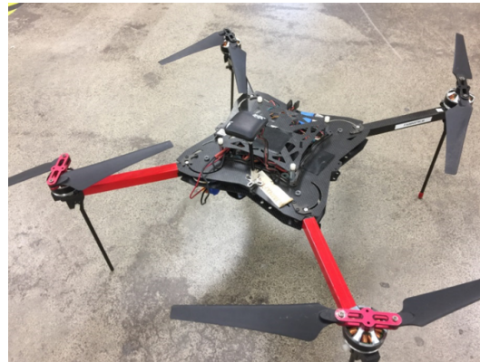
Figure 2. The Hover is equipped with a Pixhawk flight controller, GPS, telemetry antennas. Its lithium polymer battery has a capacity of 9500 mAh, which can support a 30-minute flight mission with a camera mounted on it.
