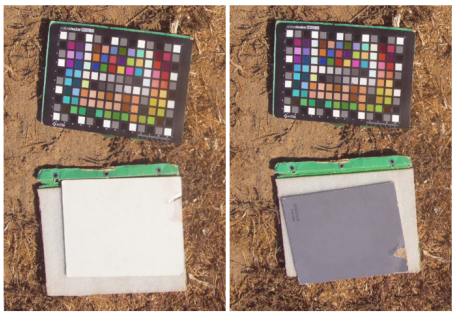
Figure 3. The images of a color panel were taken right before and after the flight missions, servicing as the reflectance reference.
