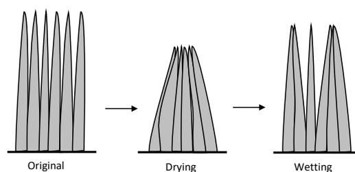
**Fig. 10** Effects of drying and wetting on the morphology of hydration products. Drying results in the collapse of needle-like structures and only partial structures can be recovered after wetting.
