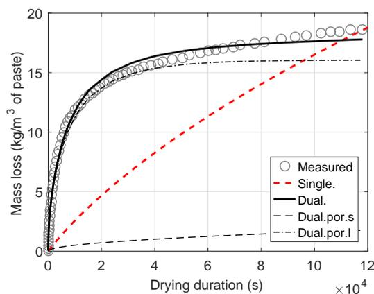
**Fig. 5** Mass loss curves for OPC paste dried at RH=80% from initially 90%.
