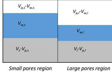
**Fig. 1** Definition of porosity in a material with two porosities. Abbreviations are:  $s$ =small pores,  $l$ =large pores,  $w$ =water occupied volume, and  $p$ =pores occupied volume.
