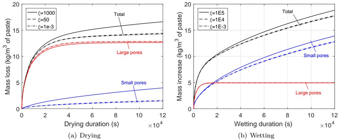
**Fig. 7** Effect of mass transfer factor on moisture transport in the specimen and in small and large pores.
