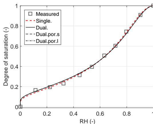
**Fig. 2** Water vapor desorption isotherms for P1 paste. The fitted curves for large and small pores are identical, so they are hidden.
