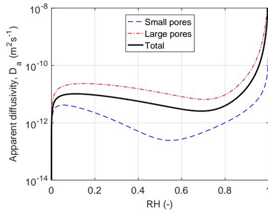
**Fig. 9** Calculated apparent diffusivity  $D_a$  (taking the case of drying at RH=80% as an example).
