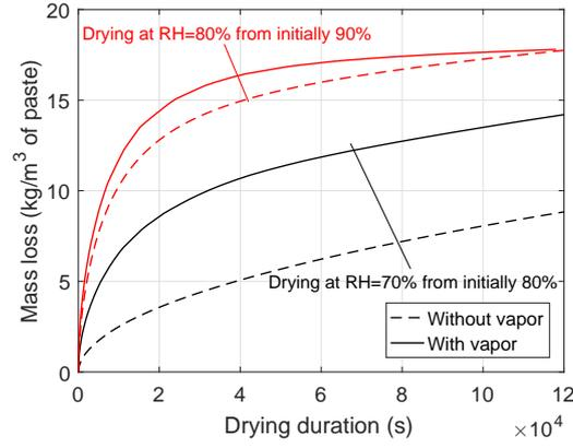
**Fig. 8** Importance to consider vapor diffusion in the dual-permeability model.
