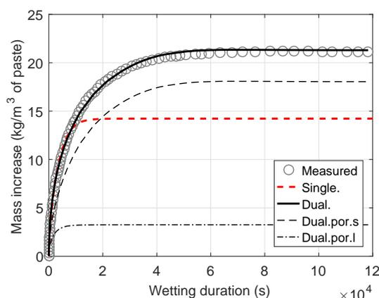
**Fig. 6** Mass increase curves for OPC paste wetted at RH=60% from initially 50%.
