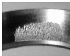
Figure 4. Outer race defect of bearing 1 of testing 2.
