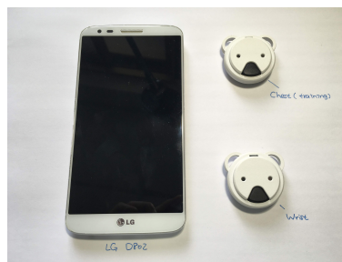
Figure 10. Required hardware in the sleep posture monitoring system. One the left is an Android smartphone, on the right are two wearable sensors.
