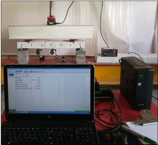
Figure 5. Typical test arrangements of segmental beams specimen
