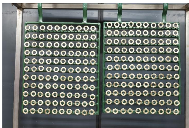
Figure 1. Galvanic frame with items placed in a fixed position.
