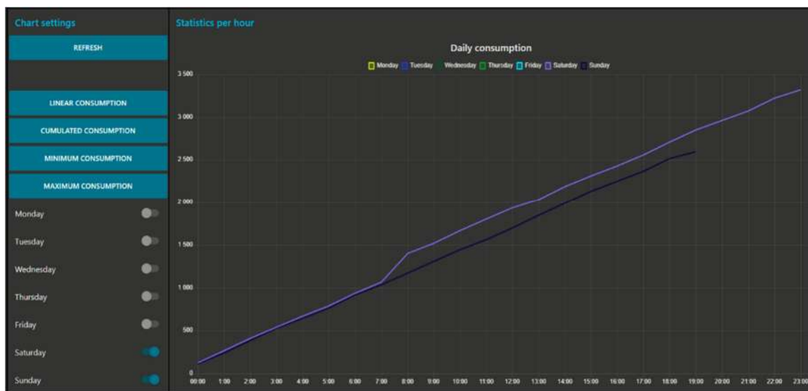
Figure 22 - Node-RED Dashboard, cumulative consumption with and without the thermal accumulator anomaly
