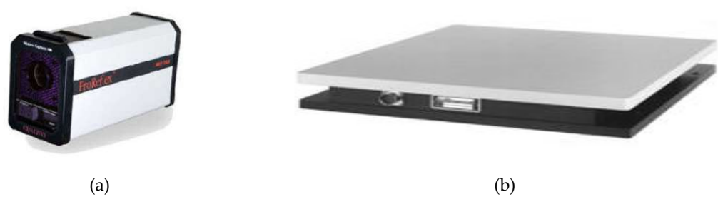
Figure 5. Measurement Equipment (a) Qualysis Motion Capture Camera; (b) AMTI force platforms.
