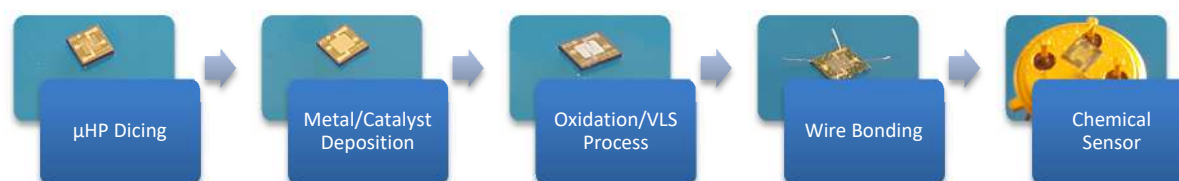
Figure 2: Flow-chart of the integration of MOX nanowires on ams \mu HPs to fabricate chemical sensors.
