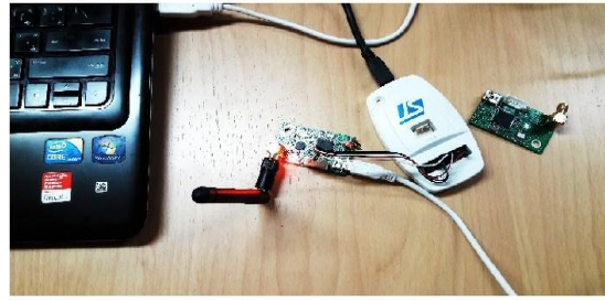
Fig. 17. A perspective of the designed sensor node accompanied by ST-Link interface.
