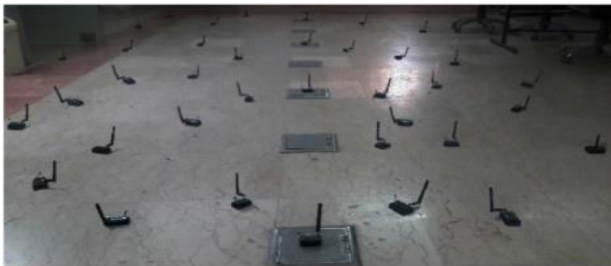
Fig. 18. A perspective of nodes distribution in indoor environment.
