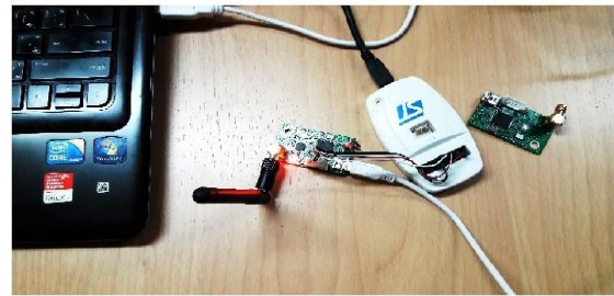
Fig. 17. A perspective of the designed sensor node accompanied by ST-Link interface.
