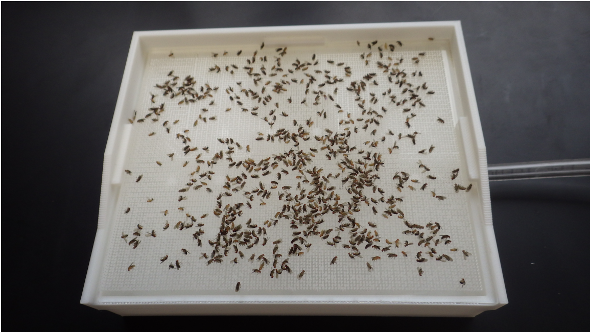
Figure 5: Photo of the assembled FLYDE plate. CO 2 is introduced to the bottom of the apparatus via the tube (on right), and dissipates through the upper plate. The tight grouping of the holes ensures that there is an ~even diffusion of gas across the surface, ensuring a consistent arena for manipulating anesthetized flies.
