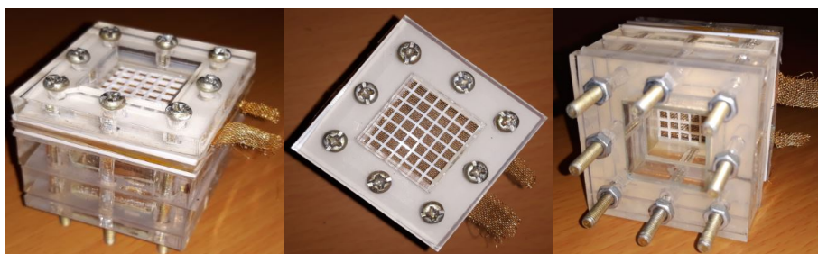
Figure 6: Schematic view of the fabricated methanol micro-fuel cell
