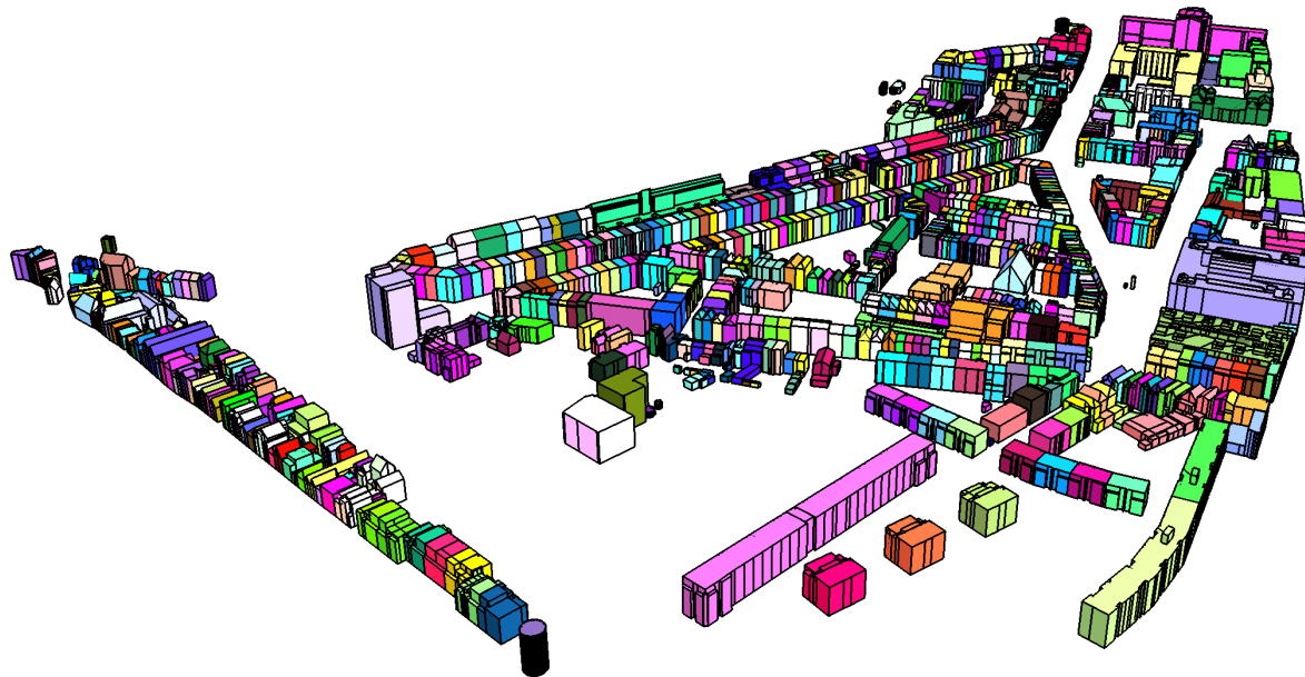
(a) Every facets (2-cells) is coloured according to the city object in the CityJSON structure. This figure proves that buildings that are merged in the same volume (3-cell) maintain their association with the original city objects.
